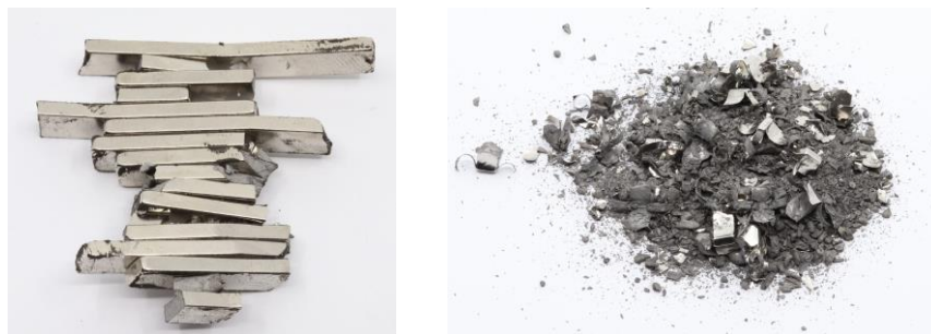
Figure 10: Nickel-coated magnets before (left) and after (right) hydrogen decrepitation.
