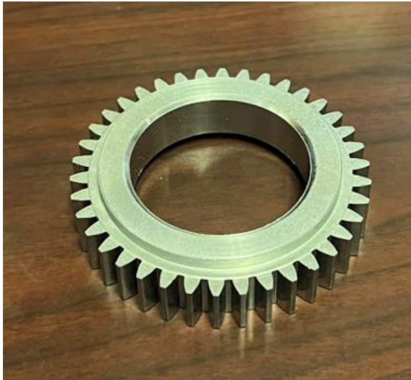
Figure 3: Representative Spur Gear Part investigated.
